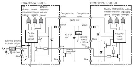
Note: The circled numbers represent the pin numbers for Pre-wired Connector Models.
