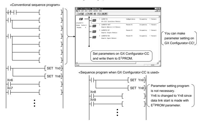
(b) Using the master parameter creating wizard, you can automatically read the loading status of remote stations and create the number of connected stations and the station information of the connected remote stations in the master parameters.
