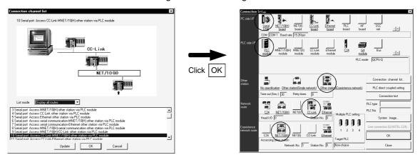
Clicking the OK button automatically sets the connection channel (areas enclosed by circles) on the Connection Setup screen.
