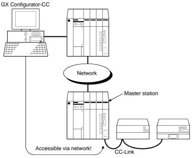
(6) You can monitor/test RX, RY, RWw and RWr You can monitor and test the RX, RY, RWw and RWr of the specified remote station.
