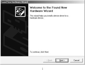
The screen shown on the left appears when you connect the personal computer and QCPU (Q mode) by the USB cable.
