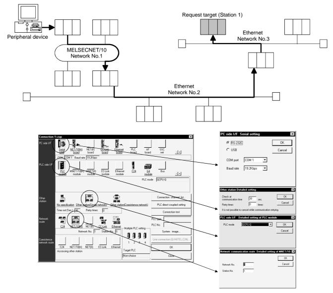
For access to the other station or multilevel system, not only the Connection Setup but also the routing parameters should be set to enable communications.
