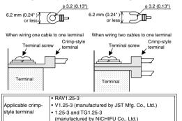
Use a crimp-style terminal in a status in which no force is applied on the cable.
