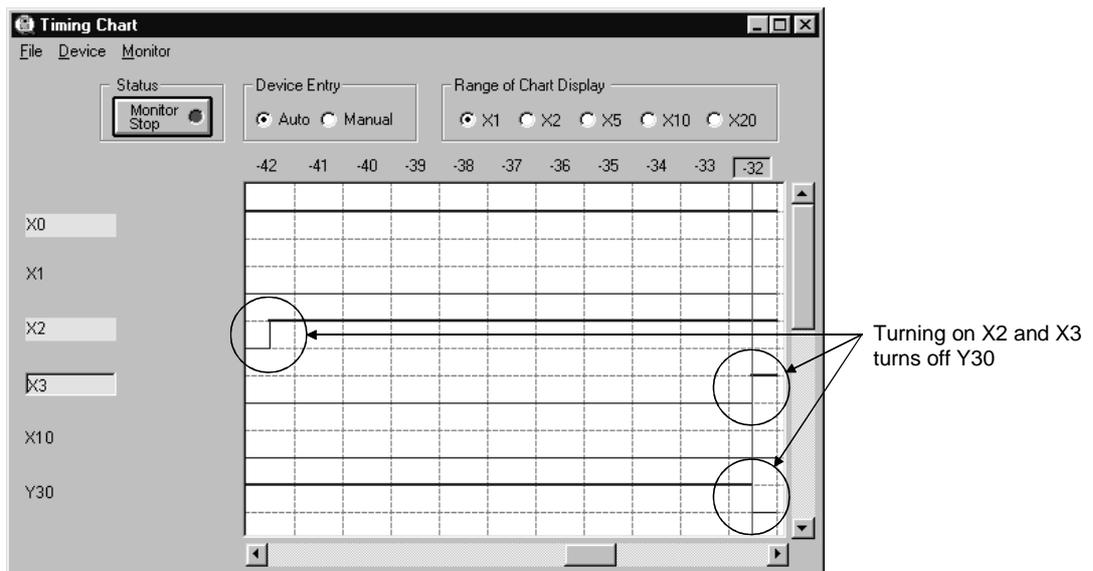
Stop monitoring and confirm the places where X2 and X3 turned on as in step 3).
