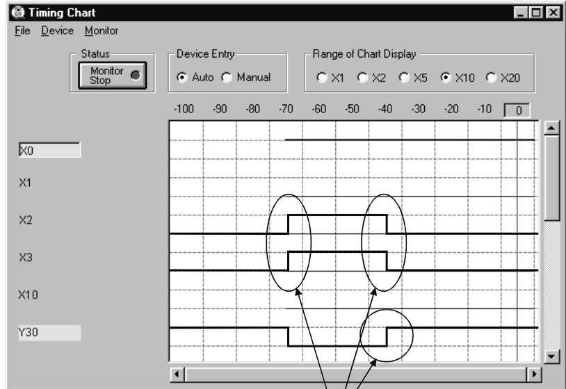
3 seconds after X2 and X3 turn on, X2 and X3 turn off and Y30 turns on
