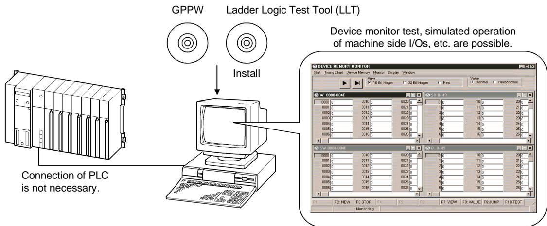
A sequence program created with GPPW can be debugged by writing it to the ladder logic test tool (LLT).
