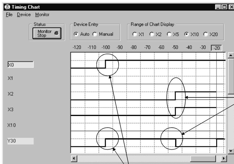
5 seconds after X0 turns on, X2 and X3 turn on and Y30 turns off
