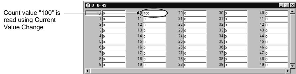
Since the sequence program uses the LED instruction to show the value on the indicator, check whether it is displayed on the basic screen.
