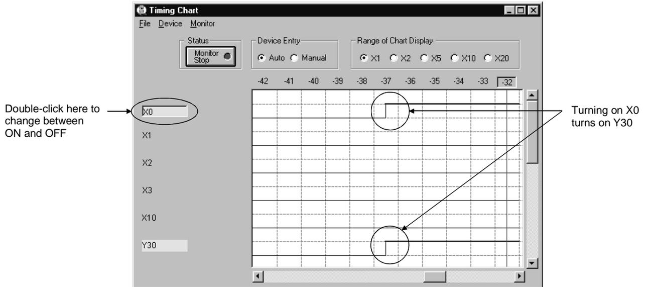
After turning X0 on, stop monitoring and move the scroll bar. When you confirm the place where X0 turned on, Y30 is on.
