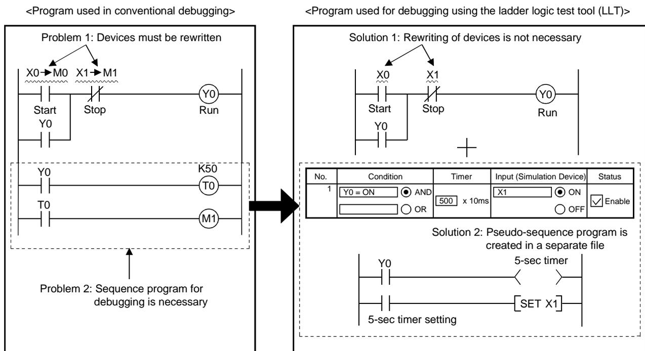
4.1 Simulation with the I/O System Setting Functions
