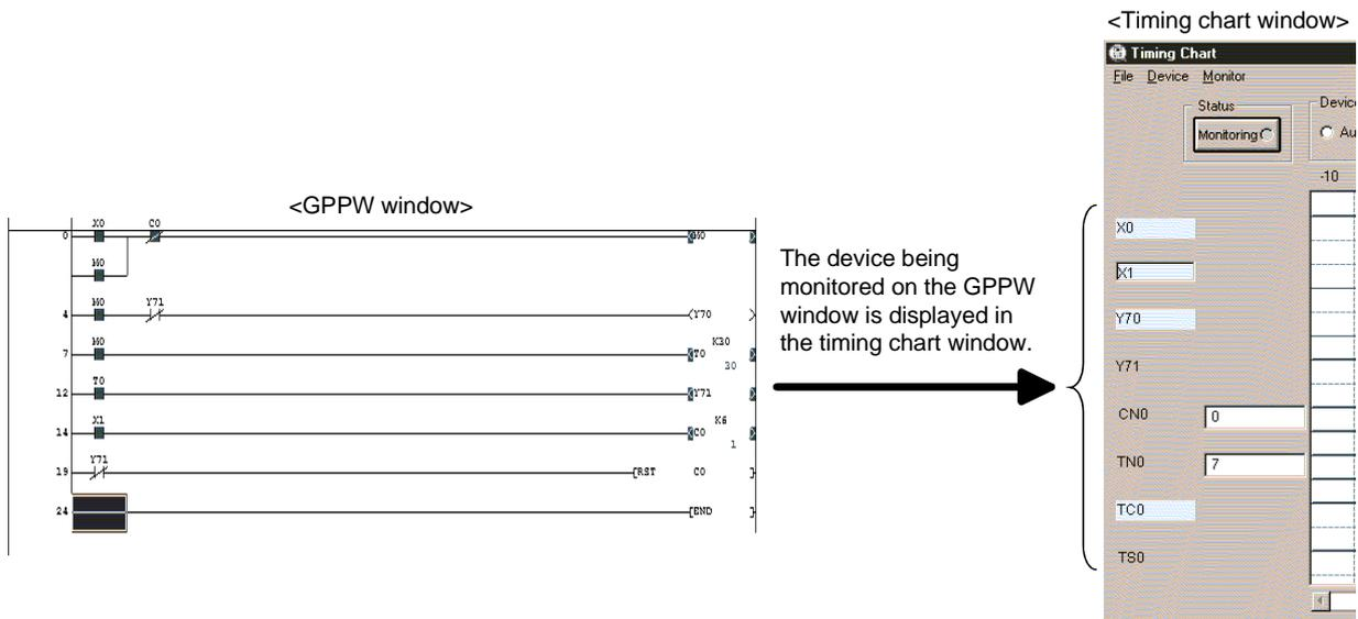
When adding a device to the registration in the timing chart window, switch the device registration setting to "Manual" after a message is displayed.
