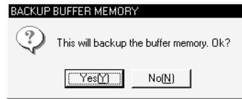
Click on the [Yes] button, to save the entire device memory or the buffer memory for the slots allocated to special function units in the I/O assignment settings.
