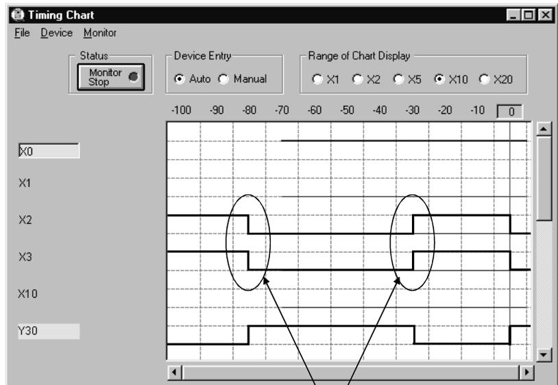
5 seconds after X2 and X3 turn off, X2 and X3 turn on
