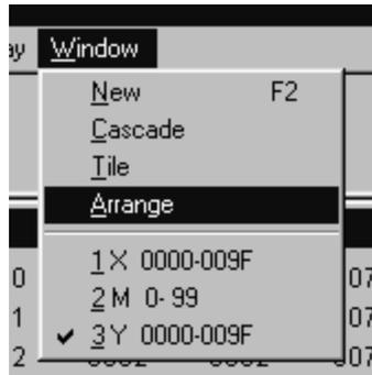
The windows reduced to icons are arranged at the bottom left of the Device Memory Monitor window.
