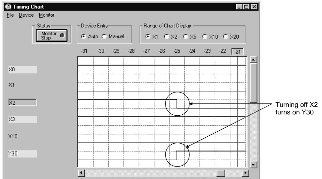
Stop monitoring and confirm the place where X2 turned off as in step 3).
