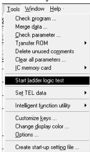
2) Click the [Tools]-[Start ladder logic test] menu of GX Developer.
