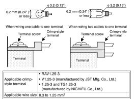
Use a crimp-style terminal in a status in which no force is applied on the cable.
