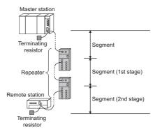
(4) Instructions for using different models of repeaters in combination Note that when combining the repeaters of different models, there are the following restrictions on the number of connectable repeaters and the number of connected stages.
