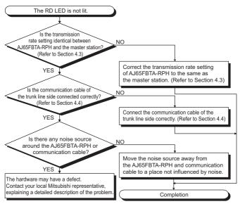
(5) The L1 to L8 RD LEDs corresponding to the data linking branch lines are not lit.
