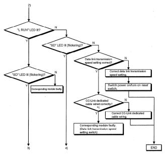
Check for short circuit, reverse connection, wire breakage, no terminal resistor, improper FG connection, improper overall distance and improper interstation distance.
