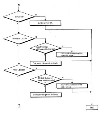
Check for short circuit, reverse connection, wire breakage, no terminal resistor, improper FG connection, improper overall distance and improper interstation distance.
