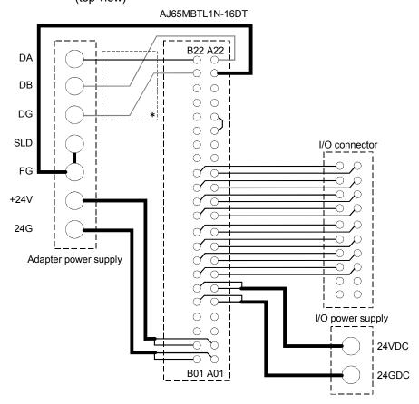
\*: When using a multi-layer board, eliminate the inner layers to prevent the capacitance between DA and DB from increasing.
