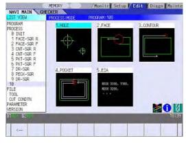
(3) Select the process mode with the cursor or the numerical value input.
