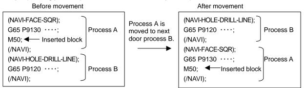
(Example2) Moving process (A inserted block exists between the processes.)
