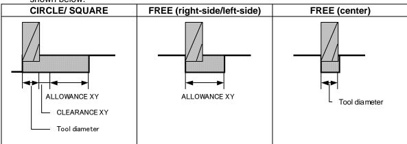
(Note) Depending on the machining pattern, the actual cutting amount of the side surfaces is differed as shown below.
