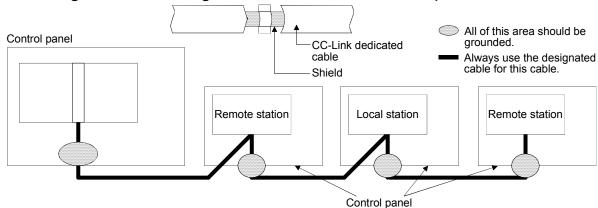
Furthermore, the grounding should be made within 30 cm (11.81 in.) of the CC-Link Ver.2 board terminal area and at the position closest to the exit of the control panel.
