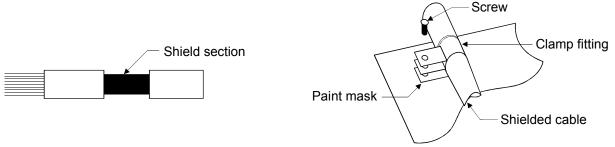
Note) The method of grounding by soldering a wire onto the shield section of the shielded cable as shown below is not recommended. The high frequency impedance will increase and the shield will be ineffective.
