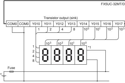
7-segment display used for sink wiring (for transistor output)
