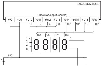
\*1 Use a 7-segment display with a latch and a built-in BCD decoder.
