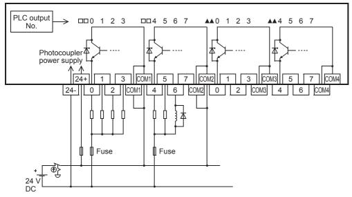
For external wiring precautions, refer to IP Page 69 Wiring precautions.
