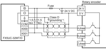
\*1 The grounding resistance should be 100  $\Omega$  or less.
