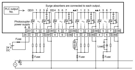
For external wiring precautions, refer to Page 75 Wiring precautions.
