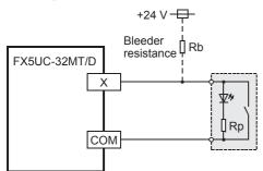
• Wiring example of FX5UC-32MT/DSS
