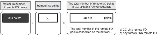
The maximum number of remote I/O points differs according to type of the network.
