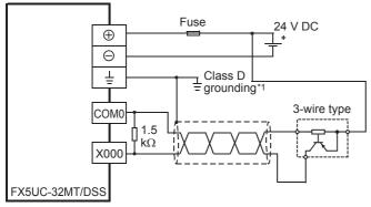
\*1 The grounding resistance should be 100  $\Omega$  or less.
