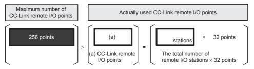
In the FX5UC CPU module, FX3U-16CCL-M parameters are set up by PLC program and will occupy up to 256 remote I/O points.
