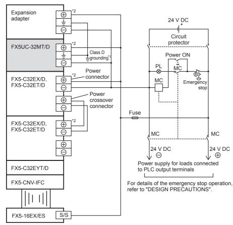
\*1 The grounding resistance should be 100  $\Omega$  or less.
