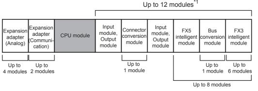
\*1 Connector conversion modules are not included in the number of connected extension devices.
