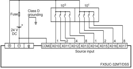
\*1 The grounding resistance should be 100  $\Omega$  or less.
