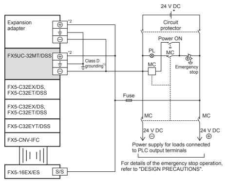
\*1 The grounding resistance should be 100  $\Omega$  or less.
