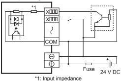
In the source input, the input (X) is turned on by connecting 24 V DC [-] with the [COM] terminal, and connecting a no-voltage contact or PNP open collector transistor output between the input terminal and 24 V DC to close the circuit.
