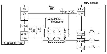
\*1 The grounding resistance should be 100  $\Omega$  or less.
