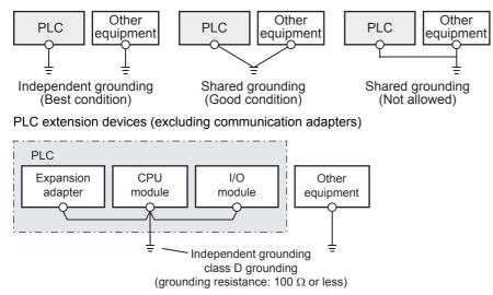
· Locate the ground point as close to the PLC as possible to minimize the length of the grounding wire.
