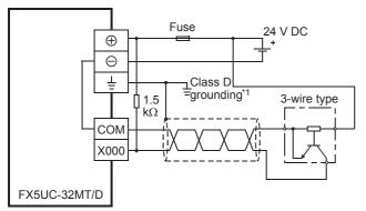
\*1 The grounding resistance should be 100  $\Omega$  or less.
