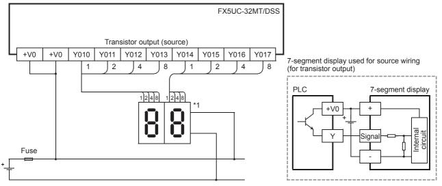
\*1 Use a 7-segment display with a latch and a built-in BCD decoder.
