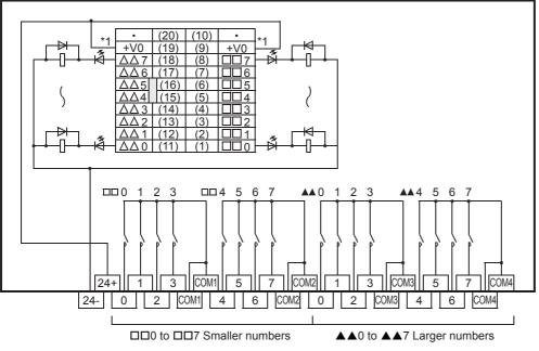
\*1 Replace this number with the one of the connected connector.
