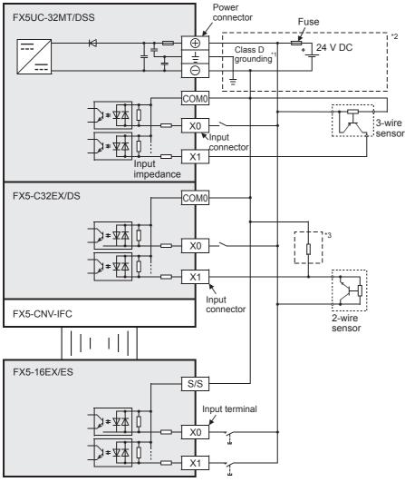
\*1 The grounding resistance should be 100  $\Omega$  or less.
