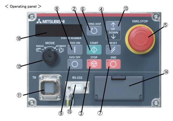
Fig.3-1: Names of controller parts
