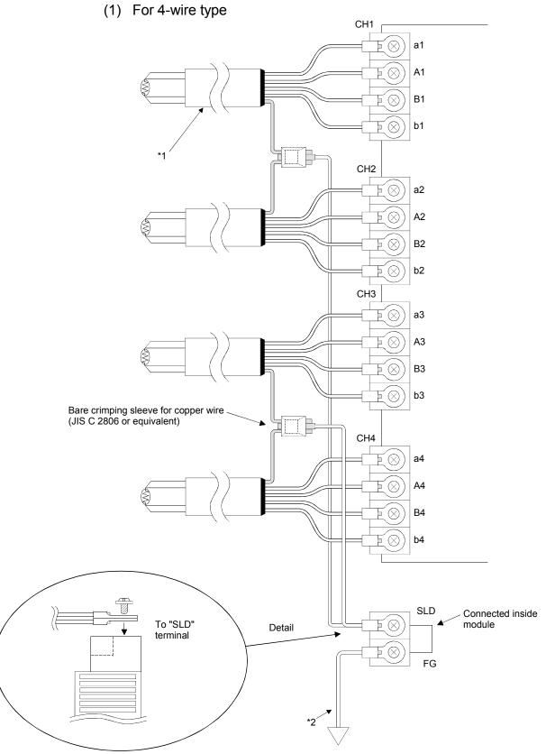
$\pm$ 1 Use the conducting cable with shield and make the wiring length as short as possible.  $\pm$ 2 Ground it to the ground terminal on the control panel.
