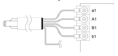
When 3-wire type is selected in switch 3 of intelligent function module switch setting
