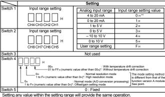
When the setting range is 1 to FH, set 1 for example Depending on the type of module used, the settings for A/D unit input range are shown below
