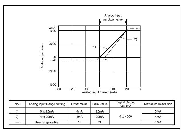
A graph of the ST1AD2-I input characteristic is shown below.
