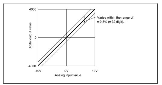
Fig. 3.3 Accuracy of ST1AD2-V
