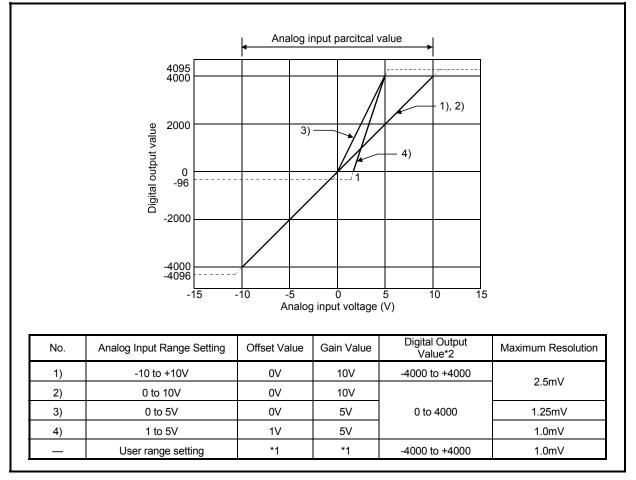
A graph of the ST1AD2-V input characteristic is shown below.
