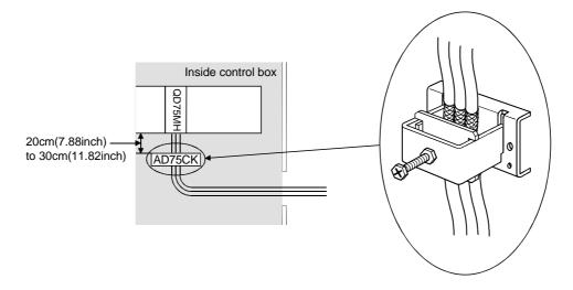
[How to ground shielded cable using AD75CK]
