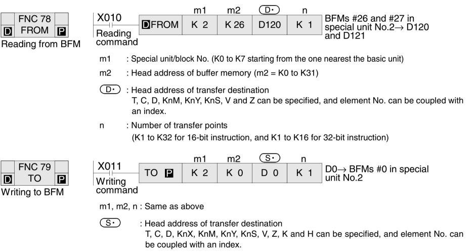
• When X010 and X011 are turned off, transfer is not performed, and data in the transfer destination is not changed. For the details, refer to the programming manual of the PC main unit.
