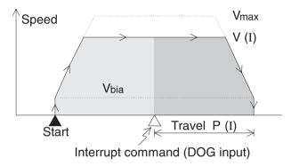
The interrupt command is connected to the DOG input in the PGU.
