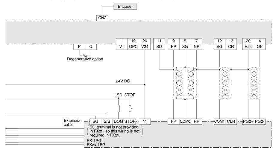
\*4 FX-1PG : Connect the VH terminal when the external power supply is 24V DC. Connect the VL terminal when the external power supply is 5V DC. Connect the FP0 and RP0 terminals with the Power Terminal for Pulse Output currently used. FX2N-1PG : Connect the VIN terminal.
