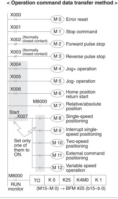
• Error can be reset by forcedly turning on/off the peripheral unit. The input X000 does not have to be used.
