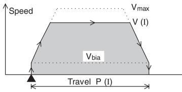
When the start command is given, the motor accelerates up to the operating speed V(I) (BFMs #20 and #19), then decelerates and stops in the set position P(I) (BFMs #18 and #17).
