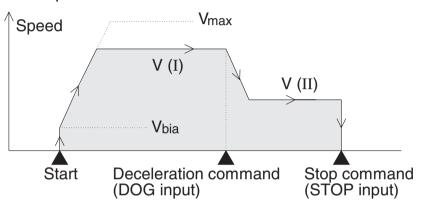
When the start command is received, the motor performs positioning at the operating speed V(I) (BFMs #20 and #19) until the deceleration command is received. At that time, the motor decelerates to the operating speed V(II) (BFMs #24 and #23). When the stop command is received, pulse generation is stopped immediately.
