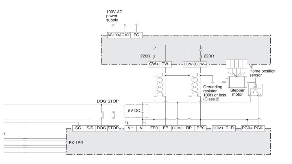
9.2 Example of Connection Between FX<sub>2N</sub>-1PG and Stepper Motor
