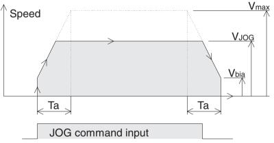
Any value between the bias speed  $V_{bia}$  (BFM #6) and the maximum speed  $V_{max}$  (BFMs #5 and #4) is valid as the command speed  $V_{JOG}$  (BFMs #8 and #7). The acceleration/deceleration time T<sub>a</sub> (BFM #15) is the time between Vbia and  $V_{max}$ .
