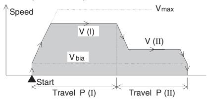
When the start command is received, the motor performs positioning at the operating speed V(I) (BFMs #20 and #19) until the set position P(I) (BFMs #18 and #17), then at the operating speed V(II) (BFMs #24 and #23) until the set position P(II) (BFMs #22 and #21) (two-step speed).
