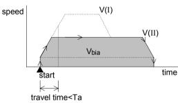
If the travel time is shorter than the time (Ta) for the PGU to accelerate to the operation speed I, the PGU operates at the operation speed II from the beginning.
