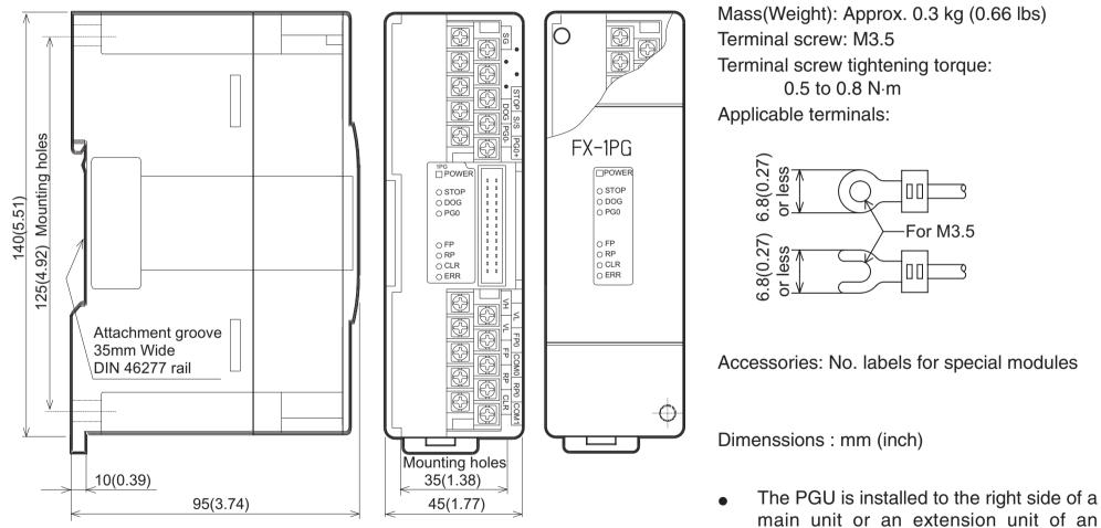
FX/FX<sub>2C</sub> Series PC or of an other extension block. The PGU can be installed using a DIN rail (DIN 46277, Width: 35 mm) or directly installed using M4 screws.
