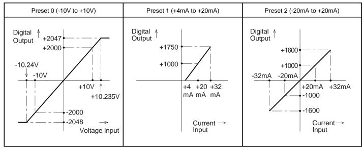
NOTE: Preset ranges are selected by an appropriate setting in buffer memory of the analog block. Current/Voltage input selection must match the correct input terminal connections.
