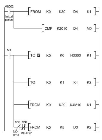
The ID code for the special function block at position "0" is read from BFM #30 of that block and stored at D4 in the base unit. This is compared to check the block is an FX-4AD, if OK M1 is turned ON. These two program steps are not strictly needed to perform an analog read. They are however a useful check and are recommended as good practise.
