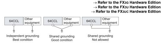
• The grounding point should be close to the 64CCL, and all grounding wires should be as short as possible.
