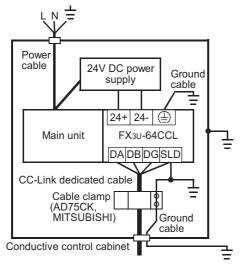
· Wiring simplified diagram
