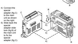
Connect all the high-speed I/O special adapters before connecting other special adapters when they are used in combination. Do not connect a high-speed I/O special adapter on the left side of a
