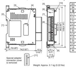
[1] DIN rail mounting groove (DIN rail: DIN46277)
