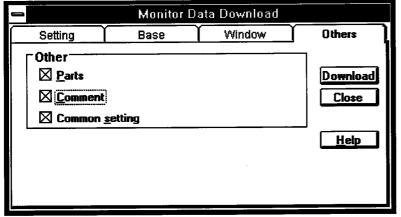
Parts data created on the screen window, part names, comments which have been created, and setting items which are common to all of the windows are downloaded here.
