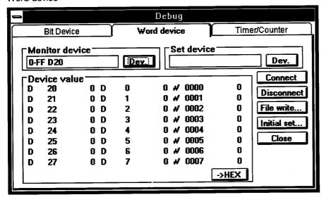
The specified device is shown at the top, in eight columns and three rows.
