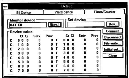
The specified device is shown at the top, in eight columns and two rows.
