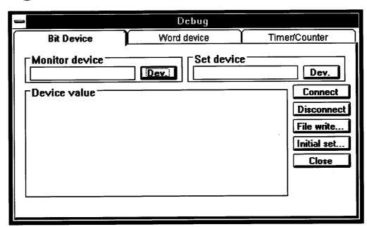
3. Clicking on Device under the "Monitor Device" parameter displays the "Device" dialog box.
