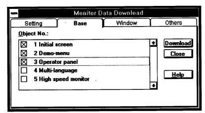
Items which were created or modified in the Base screen window are downloaded here, along with setting items which are common to all of the windows.
