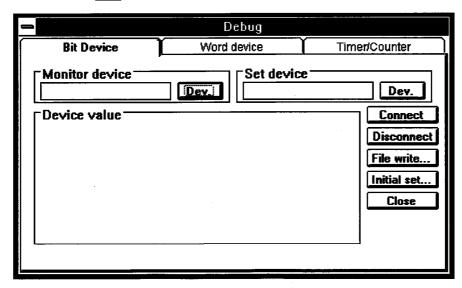
Clicking on the tab name displays the "Word device" and "Timer/Counter" debugging dialog boxes.
