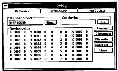
The specified device is shown at the top, in eight columns and four rows.
