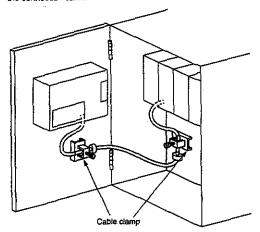
The cable clamp used by Mitsubishi Electric for the EMC specification compatibility test is shown below.
