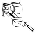
When removing the Senal Communication Module do so in reverse of the procedure shown above.
