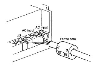
(2) When grounding a ground wire in the control panel then ground it in the same position as the LG wire and the shield mesh
