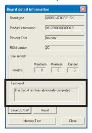
If the test completes abnormally, check the error cause on the "CC-Link IE Controller Network diagnostics result" screen of the CC IE Control utility, process the error with following the troubleshooting.
