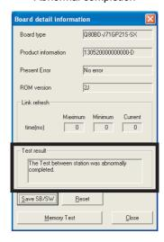
If the test completes abnormally, the cable used for the station-to-station test is faulty. Replace the cable.
