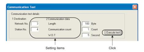
(4) When the communication test is completed, a communication test result is displayed. If an error occurs, perform the measure by following the error message.
