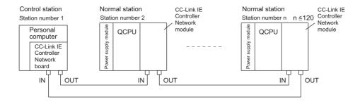
(b) Connecting the optical fiber cable
