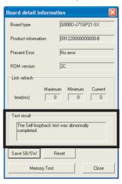
If the test completes abnormally, replace the optical fiber cable and execute the test again.
