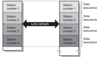
\*1: The separation prevention refers to a prevention of link data with double words (32 bits), such as the current value of the positioning module, from being separated to new data and old data in units of one word (16 bits) due to the refresh timing of cyclic transmission.
