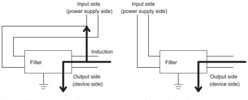
Noise will be induced when the input and output cables are bundled.
