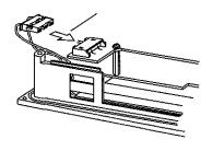
② Align the back light's left side with the display unit's back light fastener area and slide the back light into the display unit
