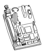
(6) Remove the back light from the display unit
