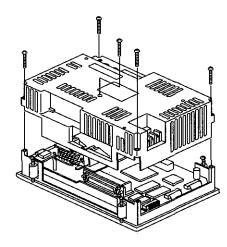
(4) Remove the back light's cable connector from the display connector
