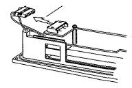
(5) Remove the back light's fastener screw with a screw driver
