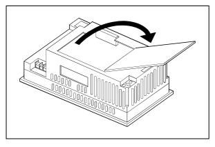
1) Open the slot cover on the back of the A956WGOT.
