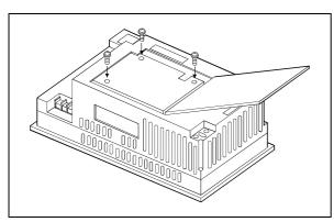
3) Fix by tightening the mounting screws of the A9GT-50WQBUSS or the A9GT-50WBUSS within the specified torque range (36 to 48 N • cm).
