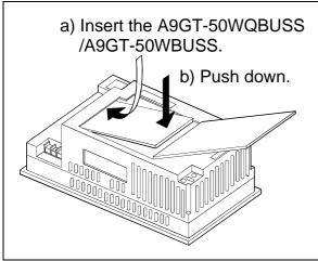
2) Mount the A9GT-50WQBUSS or the A9GT-50WBUSS in the slot for mounting a communication board. (Align the hole for the attachment screw on the transmission board with the hole for the attachment screw on the transmission board of the GOT main module, then attach.)
