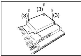
(3) Tighten and fix the mounting screws (3 pcs.) of the A9GT-BUSSU in the specified torque range.
