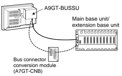
With the A9GT-BUSSU, the dimensions of the cable that protrudes from the bottom of the GOT are smaller than the A9GT-BUSS/A9GT-BUS2S type bus connection interface board (hereinafter, bus connection board) used with the conventional bus connection.
