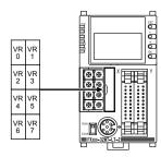
Only one analog volume expansion board can be used per main unit.
