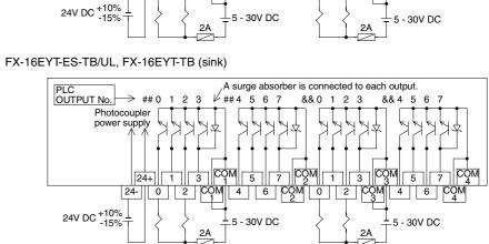
The current of 0.3 A can flow in each output point. However, in order to restrict temperature rise, flow 0.8 A to every four output points (= 0.2 A per point on an average). When turning on and off frequently a load with large rush current, set the square average current to 0.2 A or less.
