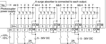
Terminal blocks are not equipped with built-in fuses. In order to prevent breakdown of circuits caused by load short-circuit, provide a fuse of 2 A for every four points.
