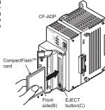
4) Close the CF card cover Set the CF card ACCESS switch to ON.
