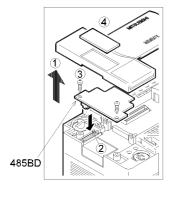
Turn off the power of the programmable controller, and mount the 485BD using the following procedure.
