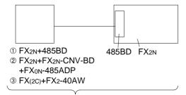
When using 485BD in system, this distance is 50m. (No use: max. 500m) But, when using FX<sub>2</sub>-40AW in system, this distance is 10m.
