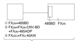
When using 485BD in system, this distance is 50m. (No use: max. 500m) But, when using FX<sub>2</sub>-40AW in system, this distance is 10m.
