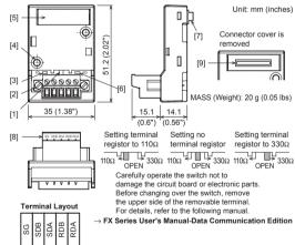
[1]Terminal resistor changing-over switch  $(110\Omega/OPEN/330\Omega)$ [2]Terminal block mounting screws
