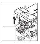
③ Fix the 232BD to the main unit using the M3 self-tapping screws provided, fitting the mounting bracket and the round crimp-style terminal with the ground cable as shown in the figure on the right. Make sure that the crimp-style terminal is attached in the direction shown in the figure on the right, and that the ground cable extends from the unit shown in the figure below. Tightening torque: 0.3 to 0.6 N•m
