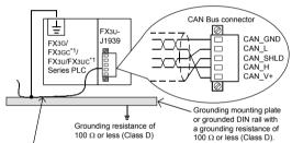
Strip a part of the coating of the shielded twisted pair cable as shown subsection 3.2.3 Ground the PLC's grounding terminal there.
