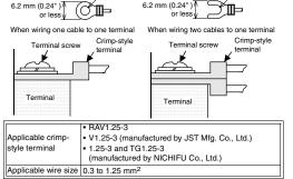
Use a crimp-style terminal in a status in which no force is applied on the cable.
