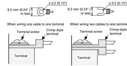
Tighten the terminal screws (M3 screws) on the terminal block with a tightening torque of 0.42 to 0.58 N·m. Do not tighten terminal screws exceeding the specified torque. Failure to do so may cause short circuit, equipment failures, or malfunctions.
