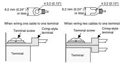
. Tighten the terminal screws (M3 screws) on the terminal block with a tightening torque of 0.42 to 0.58 N·m. Do not tighten terminal screws exceeding the specified torque. Failure to do so may cause short circuit, equipment failures, or malfunctions.
