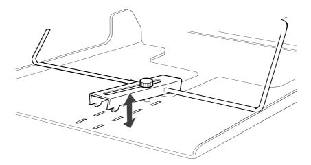
(3) Securely tighten the fixing screw.
