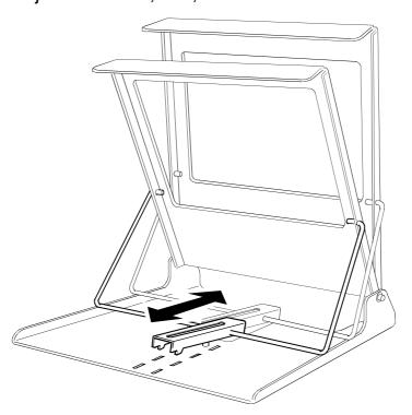
(2) Once the angle is determined, insert the angle adjustment fitting's fixing hook into the hook insertion section on the bottom of the stand.
