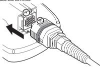
After inserting the connector, push the lock lever. The connectors are locked after the lever is pushed into
