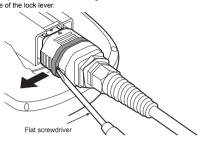
The external cable can be removed by pulling the whole plug connector while shifting the coupling of the plug connector to the cable side.
