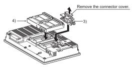
(5) Fix the CC-Link IE communication unit by tightening its mounting screws (4 places) with a tightening torgue of 0.36 to 0.48 N·m.
