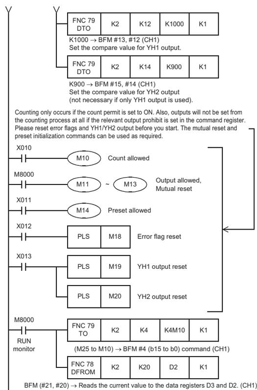
The following programs are the examples of error processing. Error status in the FX3U-2HC can be checked by reading the contents of b0 to b15 of BFM #29 to auxiliary relays of the PLC. These error flags are resettable BFM #4, #44 b8.
