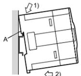
2.1.2 Direct Mounting (mounting screw: M4 screw)
