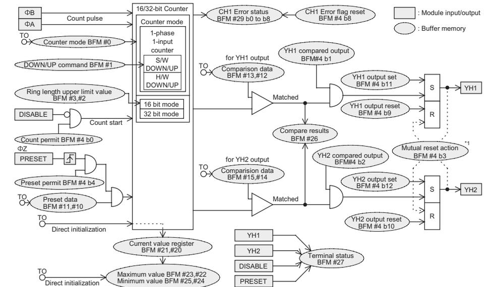
\*1 The mutual reset action becomes valid only when both the YH1 comparison output and the YH2 comparison output are permitted (BFM #4 b1, b2=ON).
