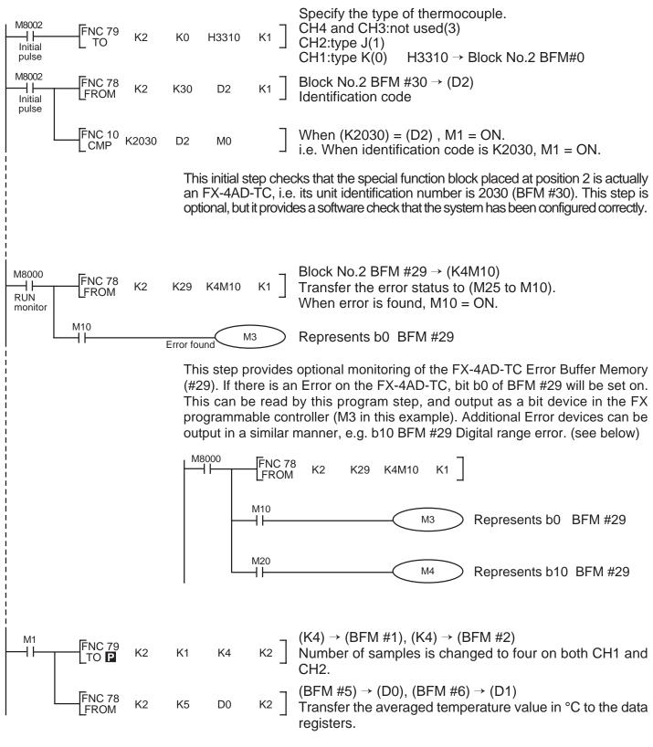
This step is the actual reading of the FX-4AD-TC input channels. It is essentially the only program step which is needed. The "TO" instruction in this example, sets the input channels, CH1 and CH2, to take the average reading of four samples.
