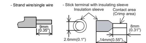
When using a stick terminal with insulating sleeve, choose a wire with proper cable sheath referring to the above outside dimensions, or otherwise, the wire cannot be inserted easily. The tightening torque must be 0.22 to 0.25 N·m. Do not tighten terminal screws exceeding the specified torque. Failure to do so may cause equipment failures or malfunctions.
