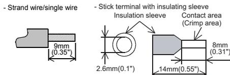
When using a stick terminal with insulating sleeve, choose a wire with proper cable sheath referring to the above outside dimensions, or otherwise, the wire cannot be inserted easily. The tightening torque must be 0.22 to 0.25 N·m. Do not tighten terminal screws exceeding the specified torque. Failure to do so may cause equipment failures or malfunctions.
