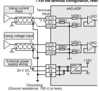
V□+, I□+, ch □: □represents the channel number \*1 Use 2-core shielded twisted pair cable for the analog input lines, and separate
