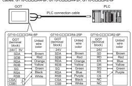
User-made cable is necessary, depending on the PLC. For the detail, refer to GOT1000 Series Connection Ma ction Manual (Mitsubishi Products) fo
