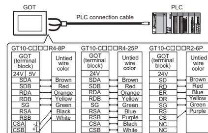
User-made cable is necessary, depending on the PLC.
