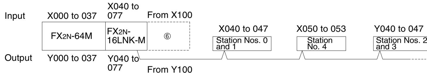
I/O assignment for remote I/O units
