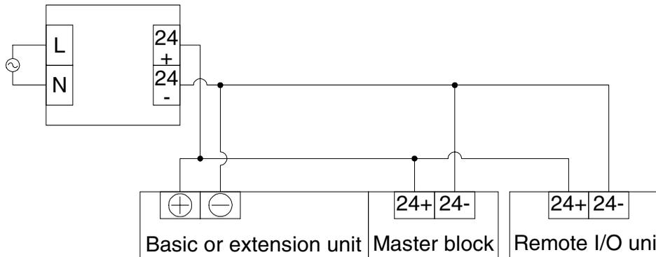
FX<sub>2NC</sub> Series (DC power supply type)
