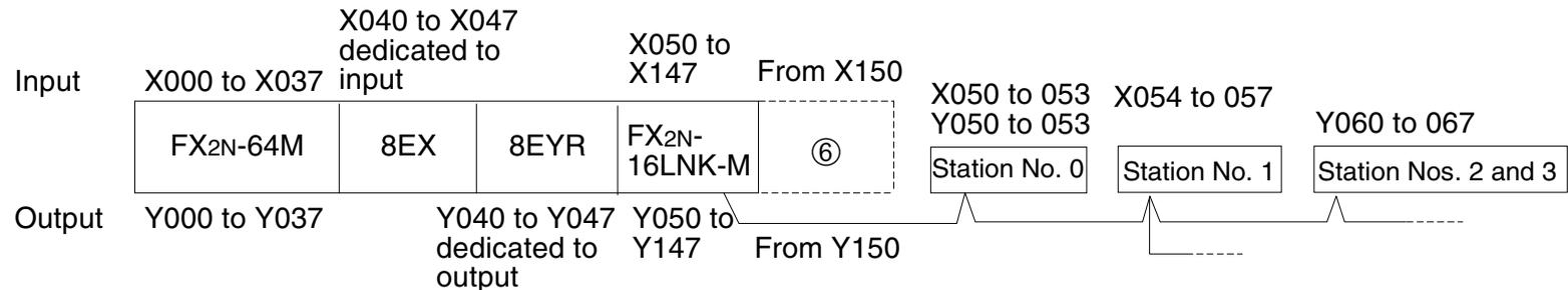
I/O assignment for remote I/O units
