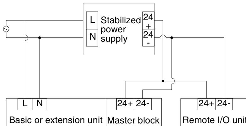
FX<sub>0N</sub>/FX<sub>1N</sub>/FX<sub>2N</sub>/FX<sub>2NC</sub>/FX<sub>3U</sub> Series DC power supply type
