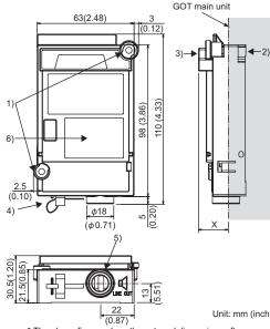
The above figures show the external dimensions after installing the cable clamp.
