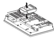
(4) Tighten the mounting screws of the sound output unit with a tightening torque of 0.36 to 0.48N•m (two
