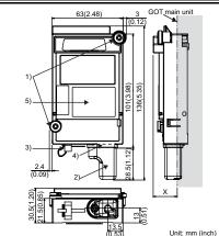
The external dimensions of printer unit with a cable clamp and connector holder attached is shown above.
